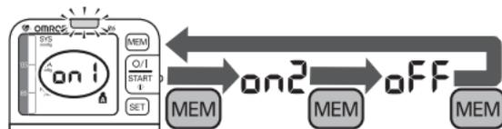
While setting the Positioning indicator the blue light flashes.
